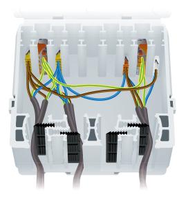
6. When a large number of cables need to be connected on a single circuit then the central receptacle can be used to connect the cable earth wires together using the 2273-108 PUSH-WIRE® connectors and jumper bar 862-482.
