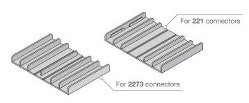
The adapters are intended to be fitted into the connector receptacles inside the WAGOBOX XLA. Each adapter provides a slot designed to hold the appropriate connector type safely and securely preventing excessive movement and inadvertent extraction of the connector or connected wire.
