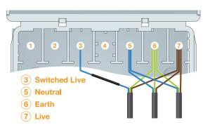
2. Prepare the cables by stripping back 70 - 80mm of the outer sheath.
