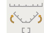
The adapters are supplied flat. To use, fold into a rectangular shape with the side fins facing inward. Insert into the connector receptacle.
